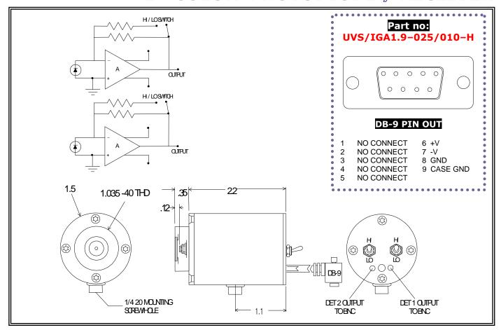
This unit is a high performance two color "sandwich" photodiode/receiver operated at ambient temperature with dual gain FET input transimpedence amplifiers. The output voltage is proportional to the input signal current:  $\mathbf{V}_{out} = \mathbf{I}_{signal} \cdot \mathbf{R}_f$ . The PD/AMPs are DC coupled dual gain systems. Care should be taken in shielding the unit from stray light during operation to prevent saturation of the amplifiers (and potential failure).
