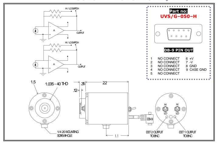
This unit is a high performance two color "sandwich" photodiode/receiver operated at ambient temperature with dual gain FET input transimpedence amplifiers. The output voltage is proportional to the input signal current:  $V_{out} = I_{signal} \cdot R_f$ . The PD/AMPs are DC coupled dual gain systems. Care should be taken in shielding the unit from stray light during operation to prevent saturation of the amplifiers (and potential failure).
