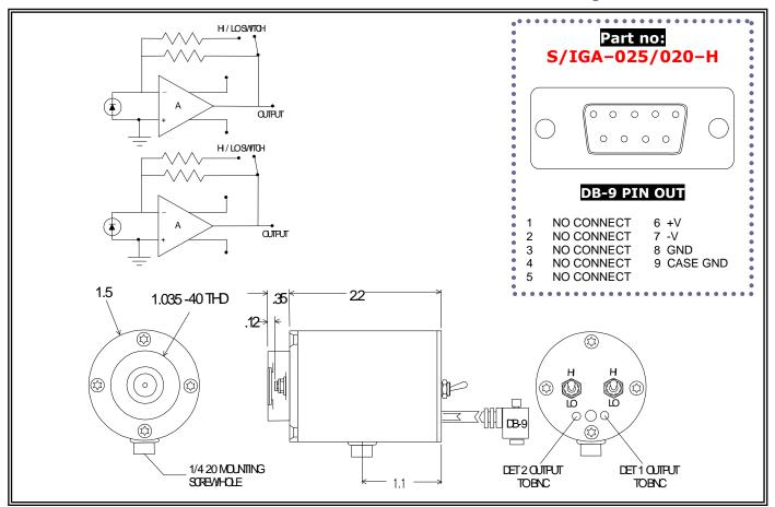
**Application** Note This unit is a high performance two color "sandwich" photodiode/receiver operated at ambient temperature with dual gain FET input transimpedence amplifiers. The output voltage is proportional to the input signal current:  $V_{out} = I_{signal} \cdot R_f$ . The PD/AMPs are DC coupled dual gain systems. Care should be taken in shielding the unit from stray light during operation to prevent saturation of the amplifiers (and potential failure).
