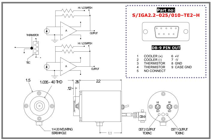
This unit is a high performance two color "sandwich" photodiode / receiver Application Note operated with a thermoelectric cooler for stabilization/cooling and dual gain FET input transimpedence amplifiers. The output voltage is proportional to the input signal current:  $V_{out} = I_{signal} \cdot R_{f}$
