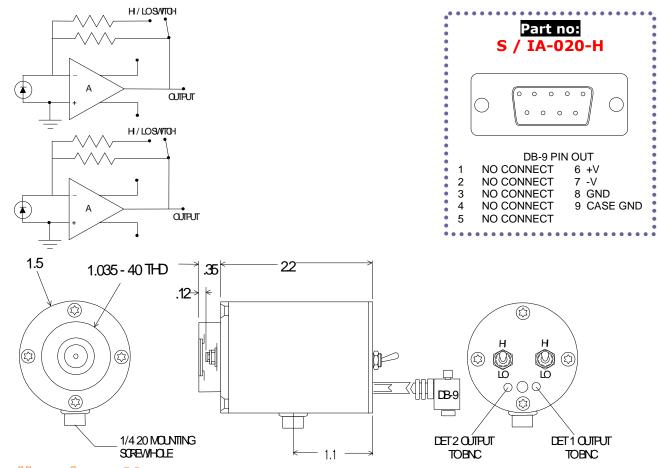
**Application** Note This unit is a high performance two color "sandwich" photodiode/receiver operated at ambient temperature with dual gain FET input transimpedance amplifiers. The output voltage is proportional to the input signal current:: Vout = Isignal R<sub>f</sub>. The PD/AMPs are DC coupled dual gain systems. Care should be taken in shielding the unit from stray light during operation to prevent saturation of the amplifiers (and potential failure).
