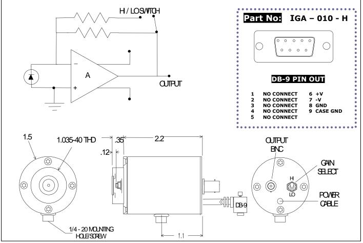
**Application** Note This unit is a high performance photodiode/receiver operated at ambient temperature with a dual gain FET input transimpedence amplifier. The output voltage is proportional to the input signal current:  $V_{out} = I_{signal} R_f$ . The PD/AMP is a DC coupled dual gain system. Care should be taken in shielding the unit from stray light during operation to prevent saturation of the amplifier (and potential failure).
